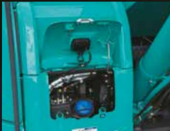
Ground level DEF tank
