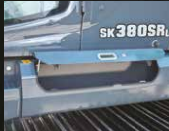
Ground level storage compartment access
