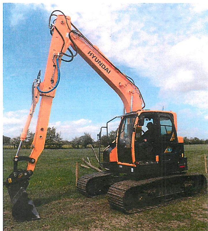
Hyundai R145LCR-9 with Sliding Dipper arm
