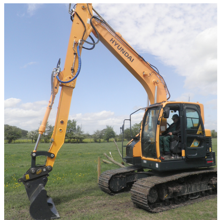
Hyundai R145LCR-9 with Sliding Dipper arm
